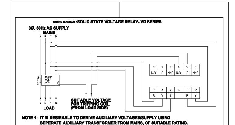
NOTE 2: FOR SHUNT RELEASE CONNECT "C" & "N/O" CONTACTS
